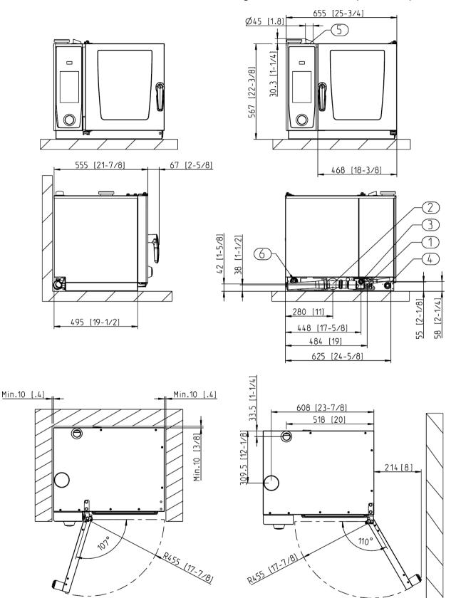
1. Common water supply (cold water) "Single" water connection as shipped 2. Drain 3. Electrical connection wire entrance 4. Chassis Ground connection 5. Steam Vent pipe 2 3/8" / 60mm 6. Splashwater-proof Ethernet socket RJ45; Minimum Clearance 2" / 50 mm Left side clearance 20" recommended for servicing of unit without the ability to move unit while connected. Measurements in mm (inch)
